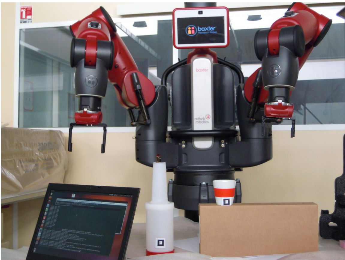
Figure 1 Baxter Research Robot equipped with parallel fingered grippers
